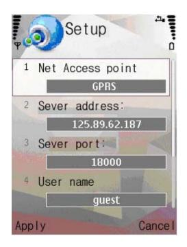
**Net Access point:** Please select the network, GPRS/EDGE/3G **Sever address:** the public IP or dynamic domain name of DVR. **Sever port:** the sever port is the mobile port you setup in DVR.
