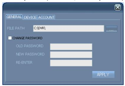
【FILE PATH】Set the location where the video or capture file is saved; 【CHANGE PASSWORD】Change the log in or the log out password of CMS.
