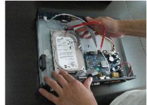
③ connect hard disk and mother board
